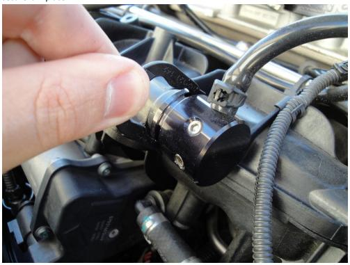
The catch tank is fitted with a sight glass on one side so you can monitor the fluid level. You will need to periodically empty this by unscrewing the drain plug on the bottom of the tank.
